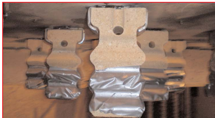
These photos show the new "top-of-the-line" ceramic hangers of the "roof" refractory repair that CORN, LP Plant Manager Andy Miller discusses in his article on page 3. The photo at left shows a close up of the metal bracket that is welded to the roof which the ceramic hanger is secured to, and the photo at right shows a series of these hangers in place.
