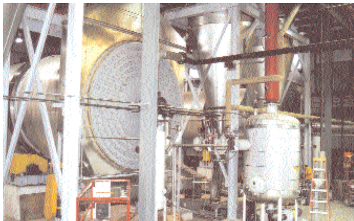
One of the three 80-foot long by 13-foot diameter steam tube dryers used to dry DDG's is pictured above.
