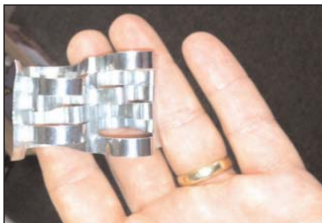
This is a picture of a media item currently being considered as a replacement option for the packing in our CO2 scrubber. The CO2 discharge stream passes through two chambers filled with similar media that are each 10 feet tall and 5 feet in diameter.
